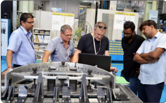
Induction of Dassault Rafale fighter jets will provide the Indian Airforce with potent multi-role, multi-mission defence capabilities. Dynamatic is building high precision assembly and conformance jigs for Dassault under the Make-in-India initiative.
