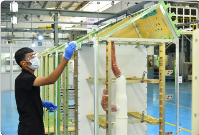
*Production of Boeing P8 - Mission Cabinets, Mechanical & Power Cabinets at Dynamic Technologies, Bangalore*
